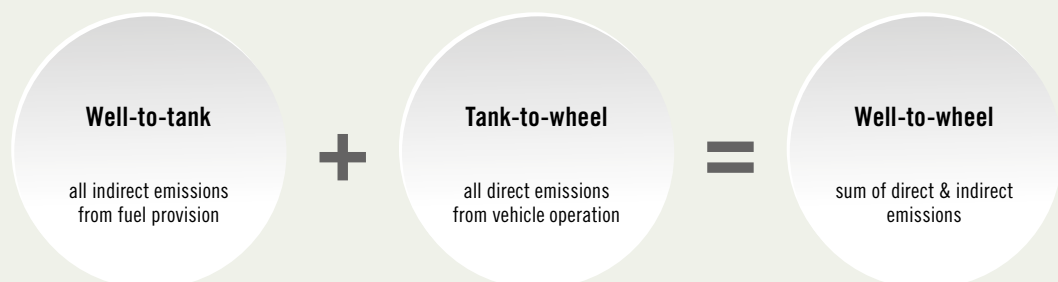
Figure: Process sections for the calculation of GHG emissions from transport services in accordance with DIN EN 16258
